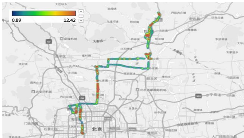
Figure 3. Concentration Distribution of Methane Along the Driving Path (ppm)
