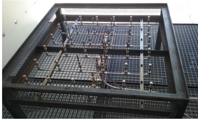
Figure 2: Picture of the 36 burner arrangement for the 1MW burner
